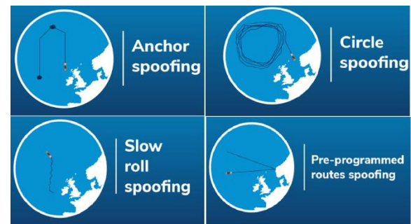
Figure 3: 4 types of AIS spoofing Source: Starboard [9]
